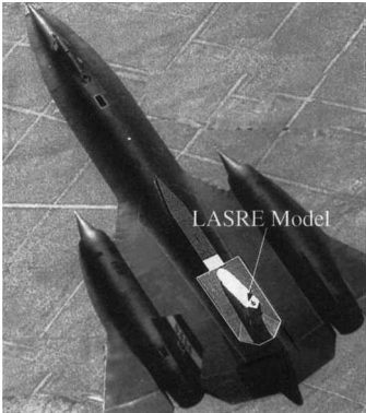
Fig. 1 LASRE experiment mounted atop the SR-71.
